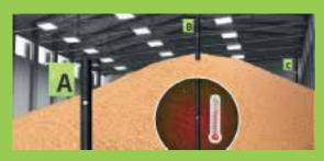
Measured values are transmitted wirelessly and are stored by the system, enabling the user to access stored data. If critical conditions are detected, the system automatically triggers an alarm via text message or e-mail.
