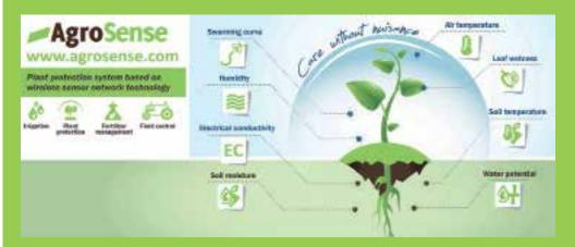
Measured values are transferred wirelessly by the system and data is centrally stored and analysed.
